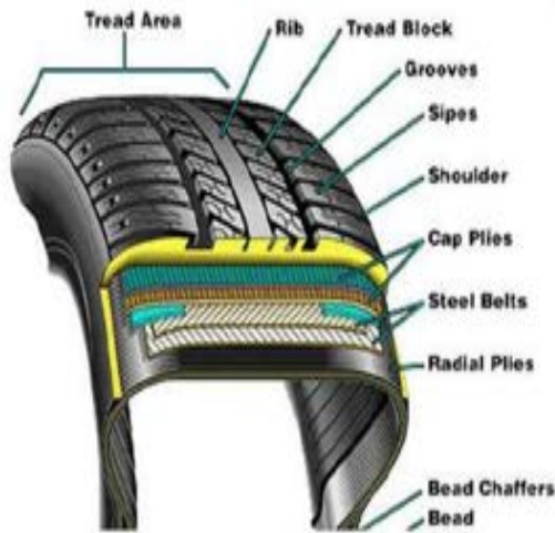
Passenger Car Tyre Cross Section
